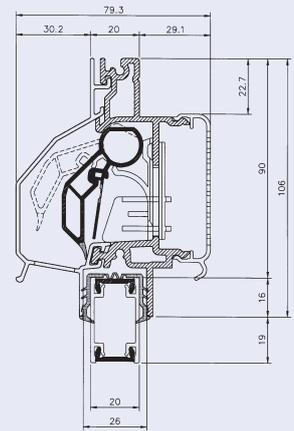
Kalfprofilen / Profils de traverse (20, 24 of 28 mm)
