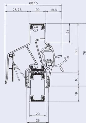
Kalfprofilen / Profils de traverse (20, 24 of/ou 28 mm)
